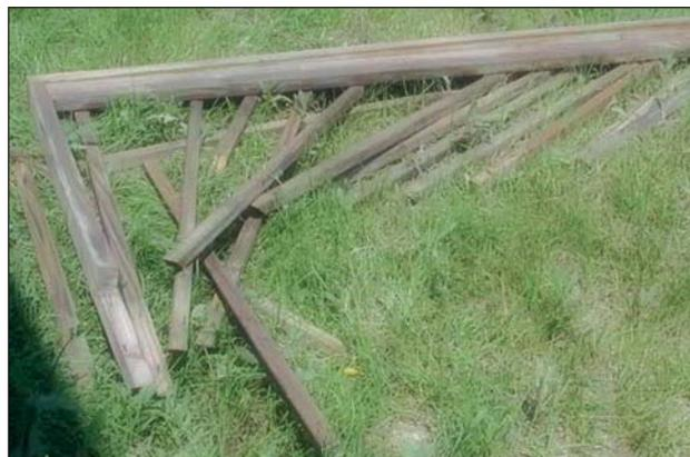
**Deadly rail.** The photo above shows an example of a grossly deficient guardrail system that produced a fatality and another injured party. In this case, a young man died after falling through the guardrail with posts that were nailed only to joists on the end of the deck. Note the notched 4x4 posts — a detail that is *not* permitted in the DCA6.
