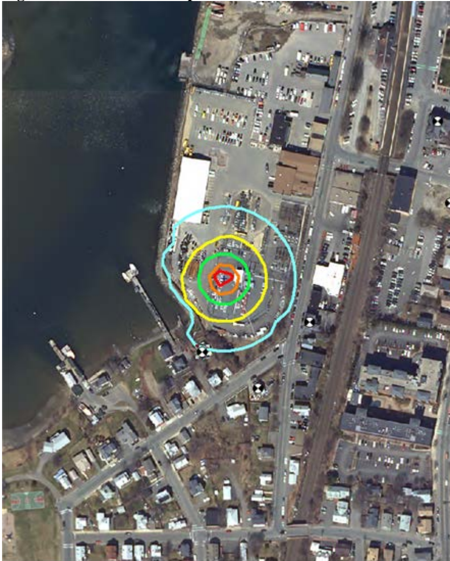
Figure 2 – Sound Level Impacts of NEMA 58 Transformer:
