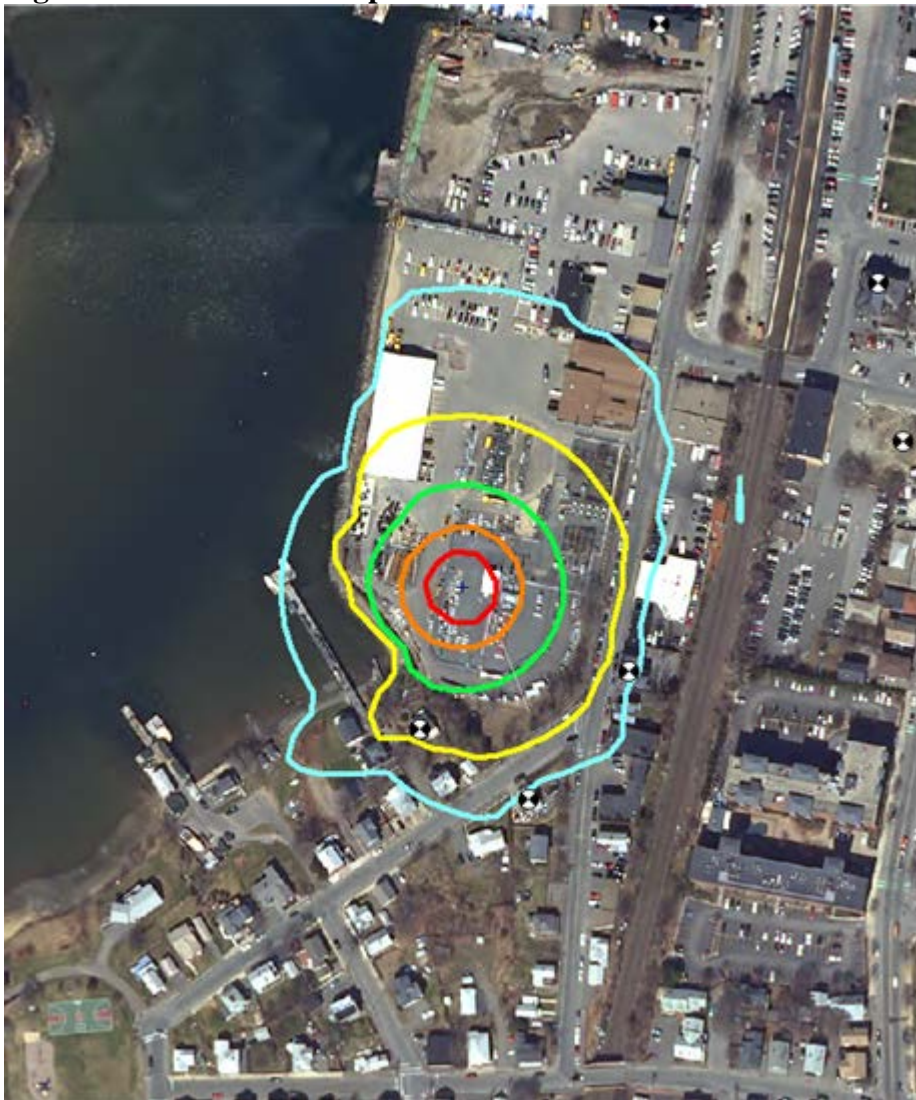
Figure 1 – Sound Level Impacts of NEMA 65 Transformer:
